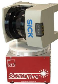
(a) One scanner configuration for 360 degree scan
