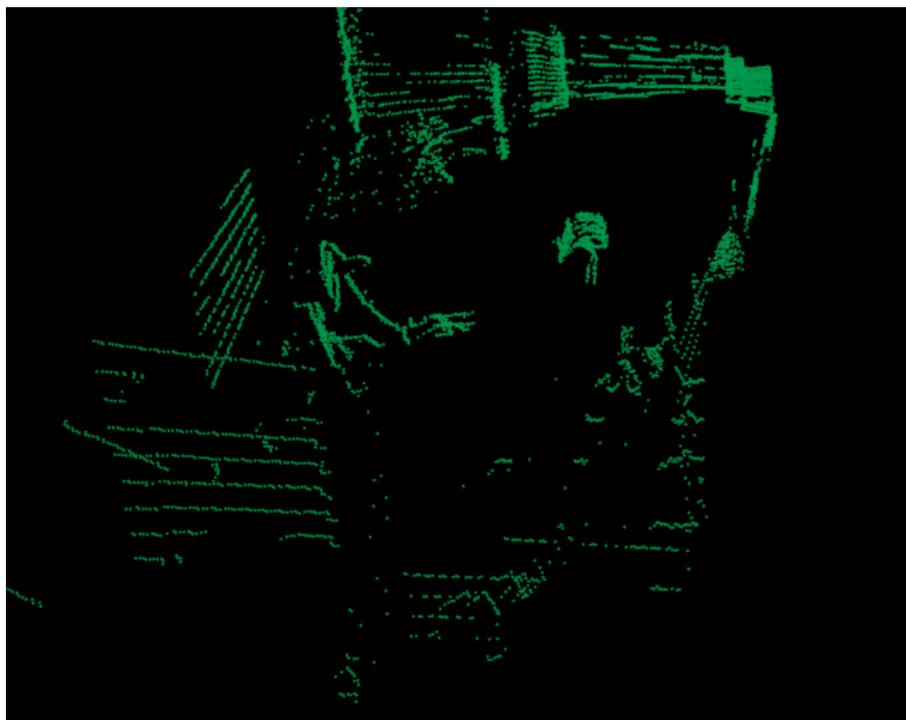
(a) Point cloud after removing 5 largest planes
