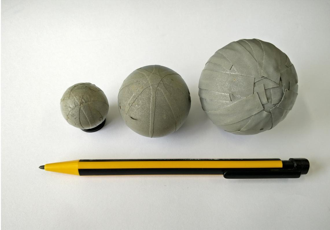
**Figure 4.2:** Artificial landmarks - The first and the third are covered with tape while the middle ball is coated with reflective paint.
